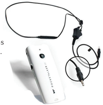
WilliamsAV Pocketalker (above) and OTOjOY's LoopBuds (below) are examples of assistive listening devices that can help reduce background noise in louder environments.
