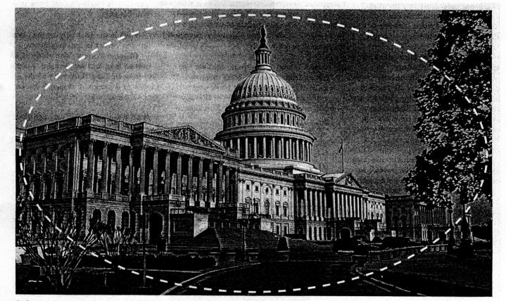
Induction loops surrounding the U.S. House and Senate chambers transmit audio pickup wirelessly to telecoils in hearing aids, turning them into in-the-ear loudspeakers for the hard-of-hearing public. Such systems can be used to enhance hearing in public buildings such as airports, courtrooms, auditoriums, theaters, shopping malls, ticket windows, churches, offices and even in automobiles so that hard-of-hearing drivers can better pick up the sounds of ambulance sirens and car horns.
